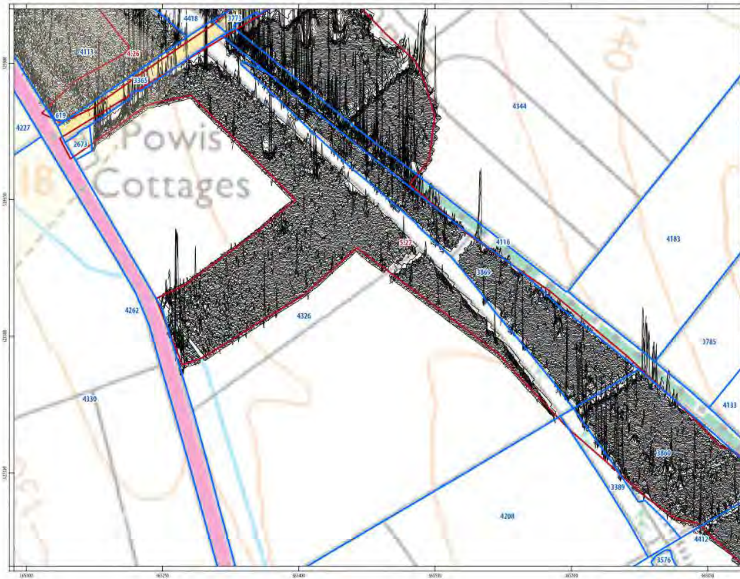
ILLUSTRATION: XY trace plot of minimally processed magnetometer data; Temple Sowerby to Appleby
