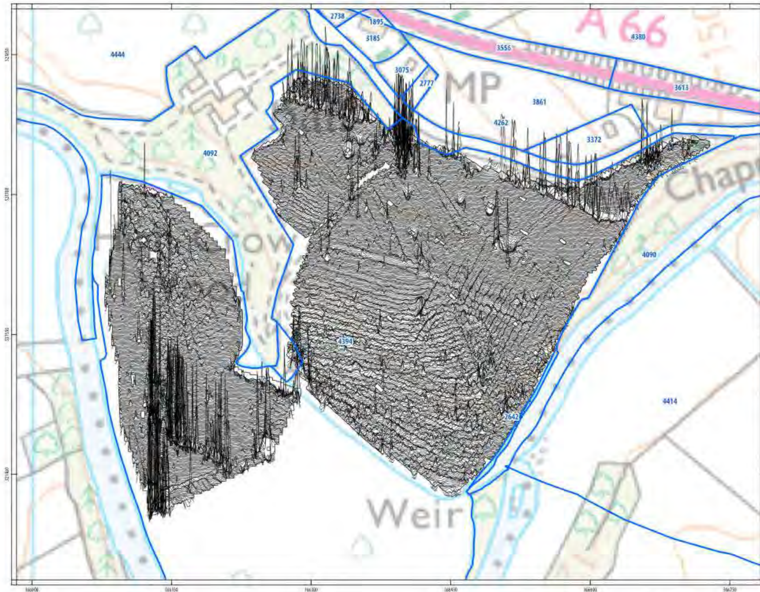
ILLUS 597 XY trace plot of minimally processed magnetometer data; Temple Saverby to Appleby
