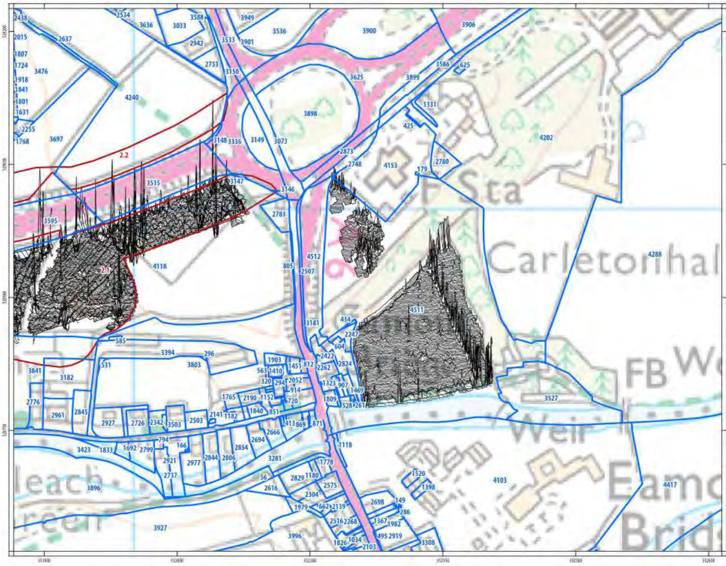
ILLUS 587 XY trace plot of minimally processed magnetometer data; M6 Junction 40 to Kemplay Bank Roundabout
