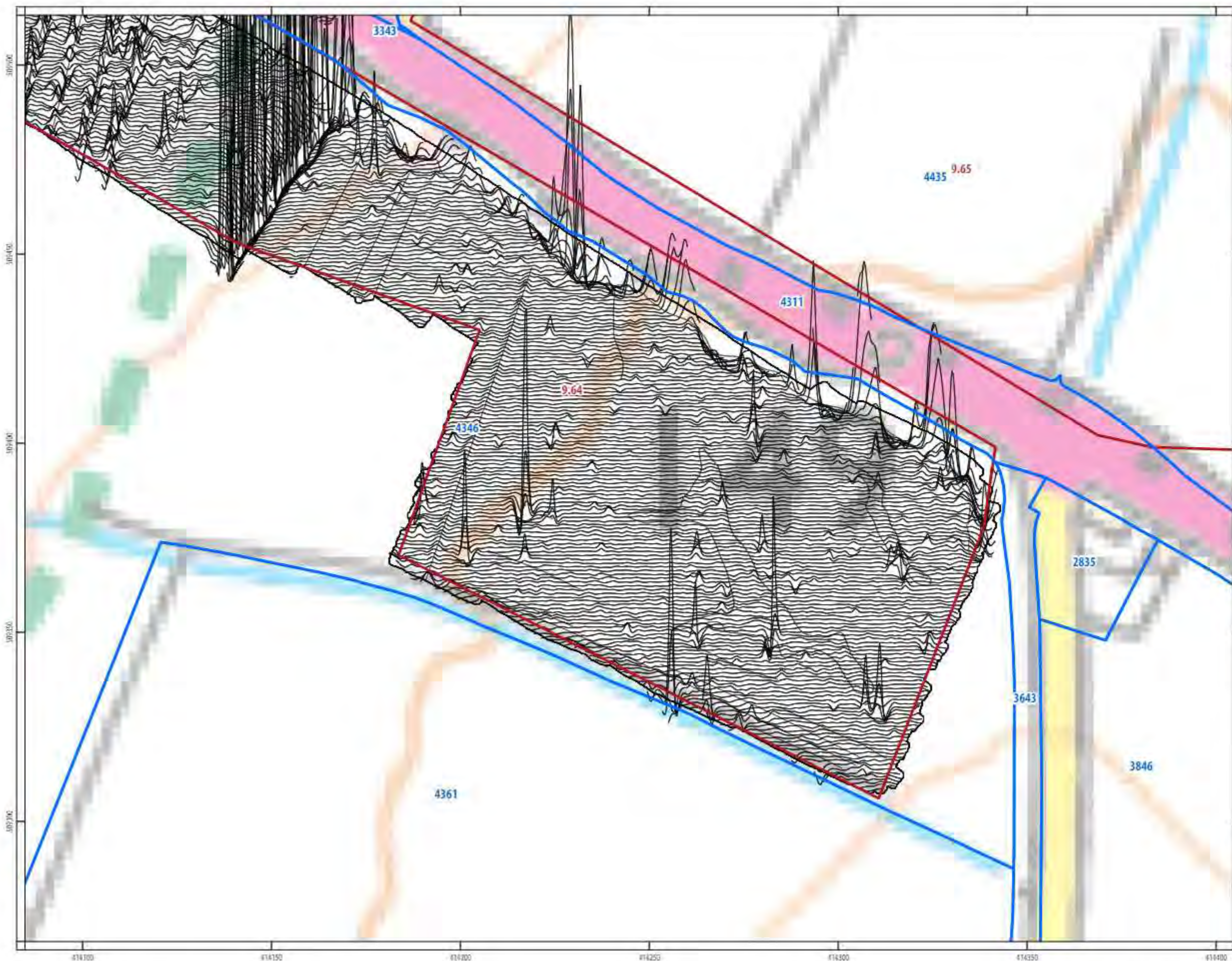
ILLUS 324 XY trace plot of minimally processed magnetometer data; Stephen Bank to Carkin Moor
