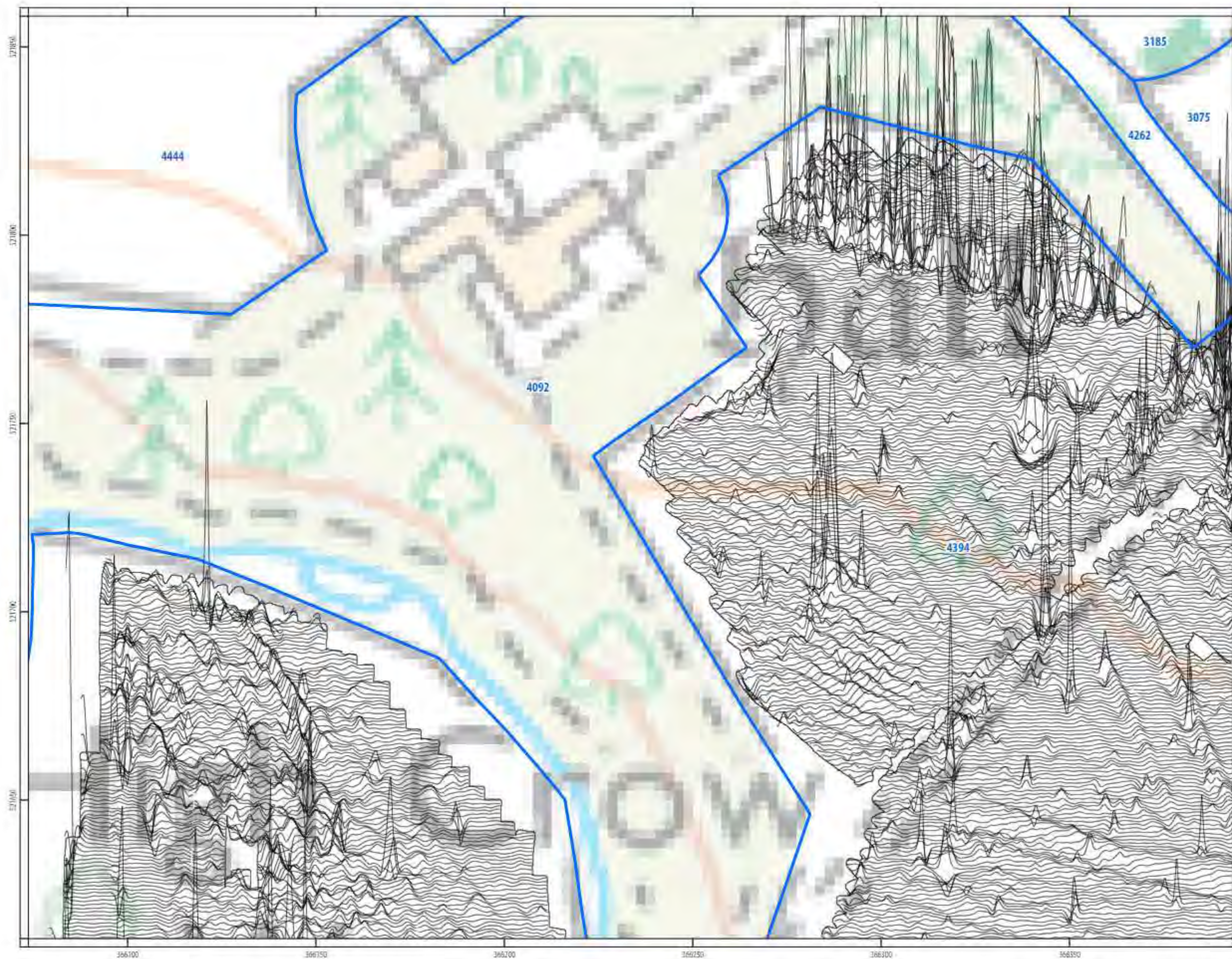
ILLUS 646 XY trace plot of minimally processed magnetometer data; Temple Sowerby to Appleby
