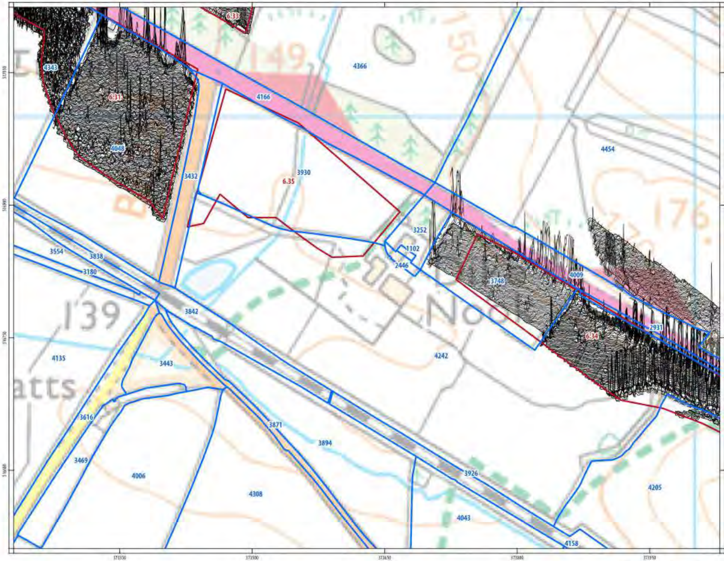
ILLUS 198 XY trace plot of minimally processed magnetometer data; Appleby to Brough (Warcop)
